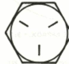
Drawing to the left is of the head of a harden steel bolt. Note the three lines on the top of the head which denote harden steel.
