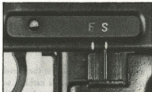
Upper left: semi-auto Uzi select lever, note only two position, in safe position. Lower right: full-auto Uzi three position select lever in repetition (semi) position.
