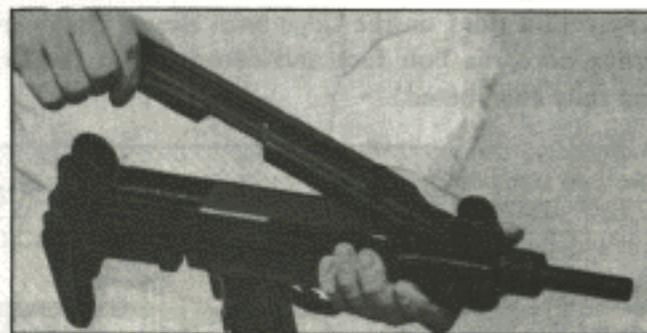
1. Press the cover catch to the rear (located in the fore part of the rear sight seating), raise the rear part of the cover and remove to the rear and upwards. This frees it from the body of the gun.
